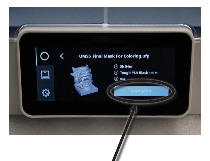
NOTE: Both the extruder and the build platform may be very hot immediately after the print finishes. These components can burn you if you touch them. Therefore, wait a short period of time before removing your print. Doing so will help substantially when you remove your print from the build platform
