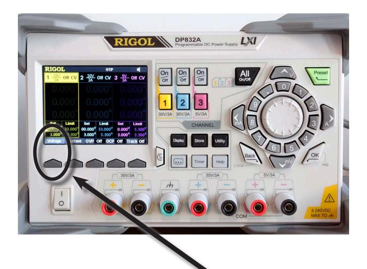
4. Using the number buttons on the button wheel, enter the voltage you want (i.e. 5.0V)
