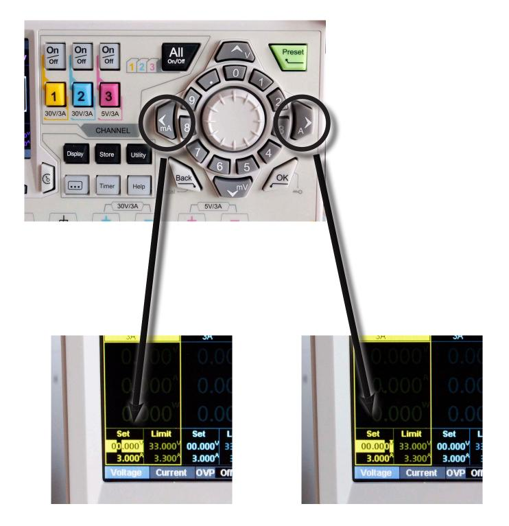
5. Rotate the dial to increase/decrease the voltage for that digit (i.e. 5.000 for 5V)
