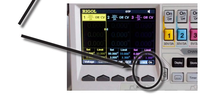
3. Select Channel 1 (Note the "link" icon on the screen connecting channel 1 and channel 2)
