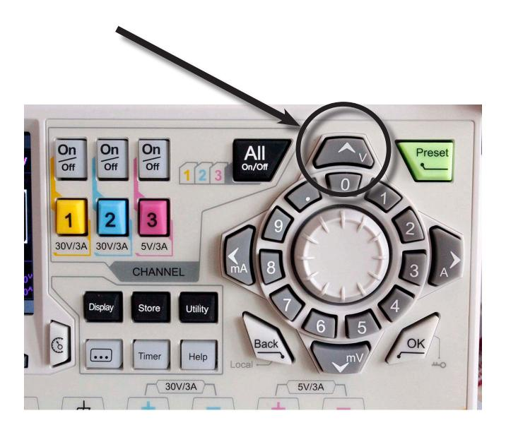
5. To engage the OVP, press the OVP soft key again. (It will say ON). If you accidentally exceed your voltage limit, the OVP will automatically turn off that channel.
