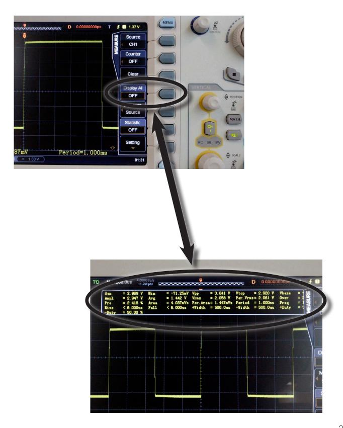
21. The trigger is set to "auto" by default. You can adjust the trigger level by rotating the trigger dial
