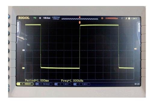
12. You can change the horizontal position by rotating the horizontal position dial. (Note the green arrow move as you rotate)
