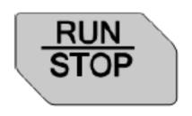
Press this key to set the state of the oscilloscope to "RUN" or "STOP". In "RUN" state, the key is illuminated in yellow and red in "STOP" state.
