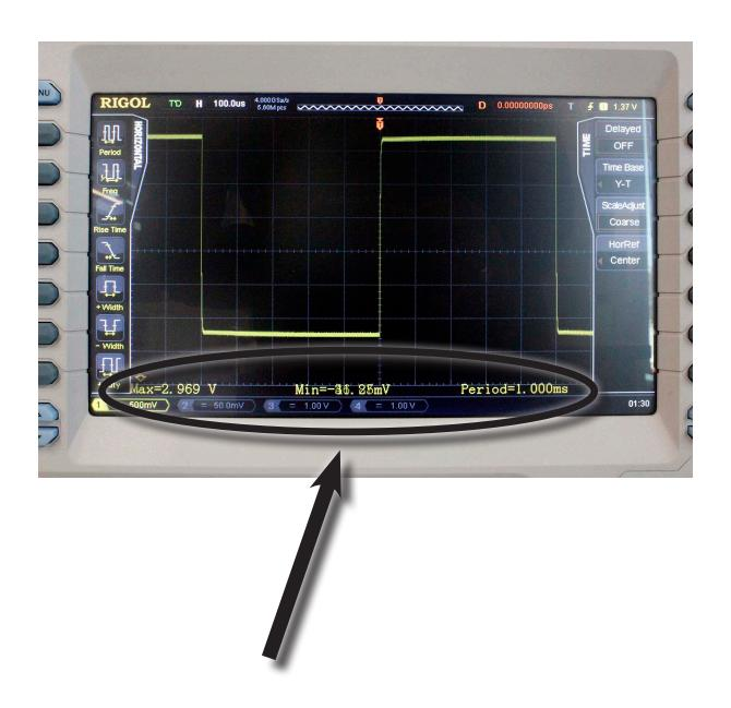
19. To display all information about your waveform, press the "Measure" button on the front panel
