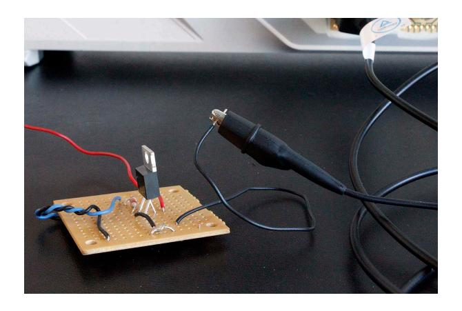
4. Connect the probe's measuring clip to the point within your circuit you wish to measure
