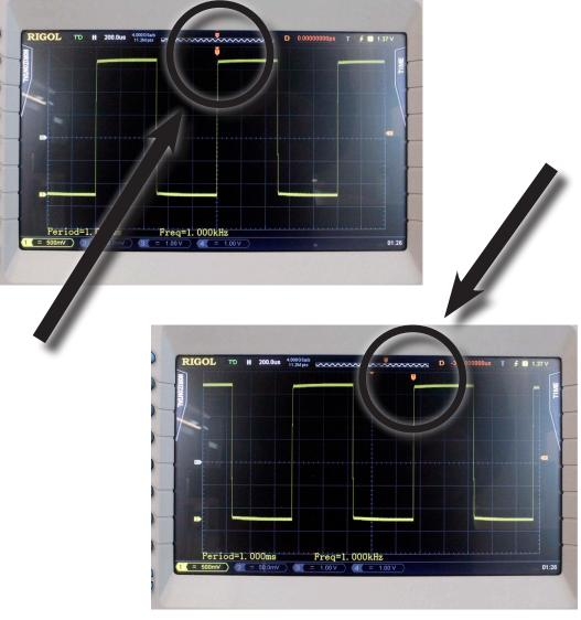
13. To return to the original position, press the horizontal position button
