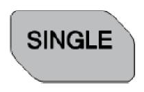
Press this key to set the trigger mode to "Single". In single trigger mode, the oscilloscope generates a trigger when the trigger conditions are met and then stops. When the oscilloscope is in waitfor-trigger state (the key is illuminated in orange), pressing FORCE will generate a trigger signal immediately.
