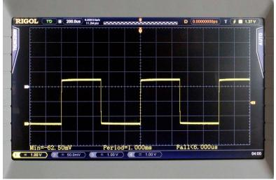
15. To change the vertical position, rotate the vertical position dial. (Note the green arrow move as you rotate)
