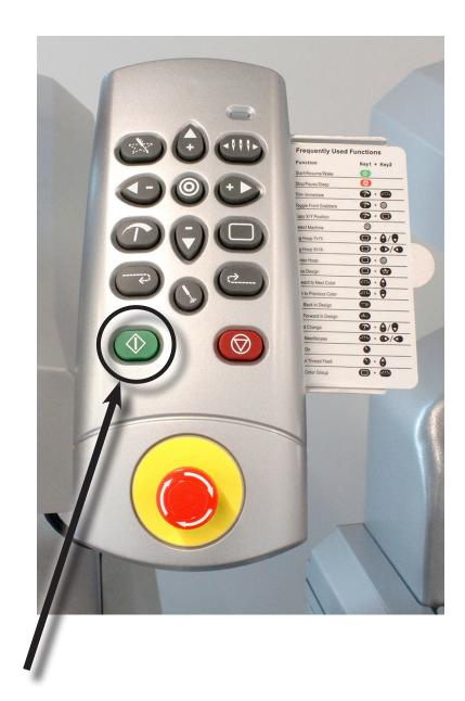
15. If there is a thread/bobbin break, the machine will stop. Ask one of the shop staff to assist you if this happens. After the issue has been corrected, use the Jog button on the controller pendant to return to the last successful stitch. (The laser pointer will help locate this)
