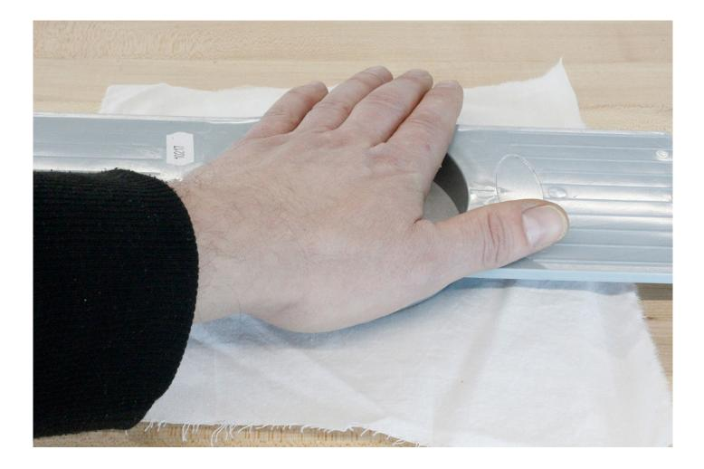
9. Once the hoop is seated, tighten the tension screw on the hoop-ring
