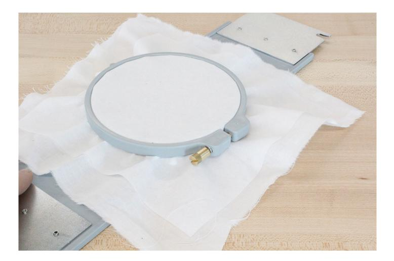
10. Pull the fabric tight and flat. It should sound like a small drum when you tap your finger on it. Failure to ensure the fabric is taught and flat will result in a failed job.
