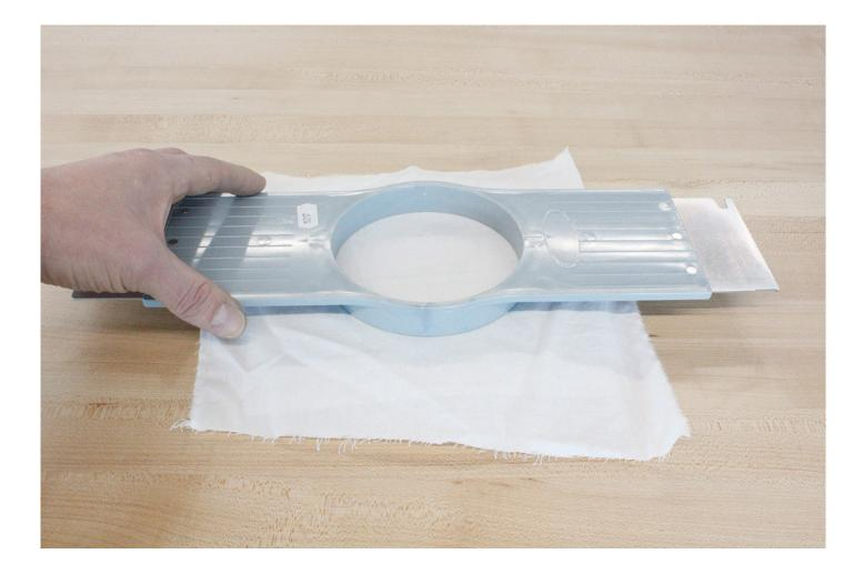
7. Using the mounting brackets as a guide, make sure the hoop is centered and level on the fabric correctly.
