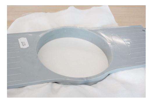
11. Check the back of the hoop to ensure there are no wrinkles or other parts of the fabric lodged in the hoop
