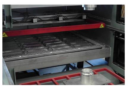
7. Open the safety gate and secure your Die in the lower platen fixture. Be mindful to not overtighten the screws.
