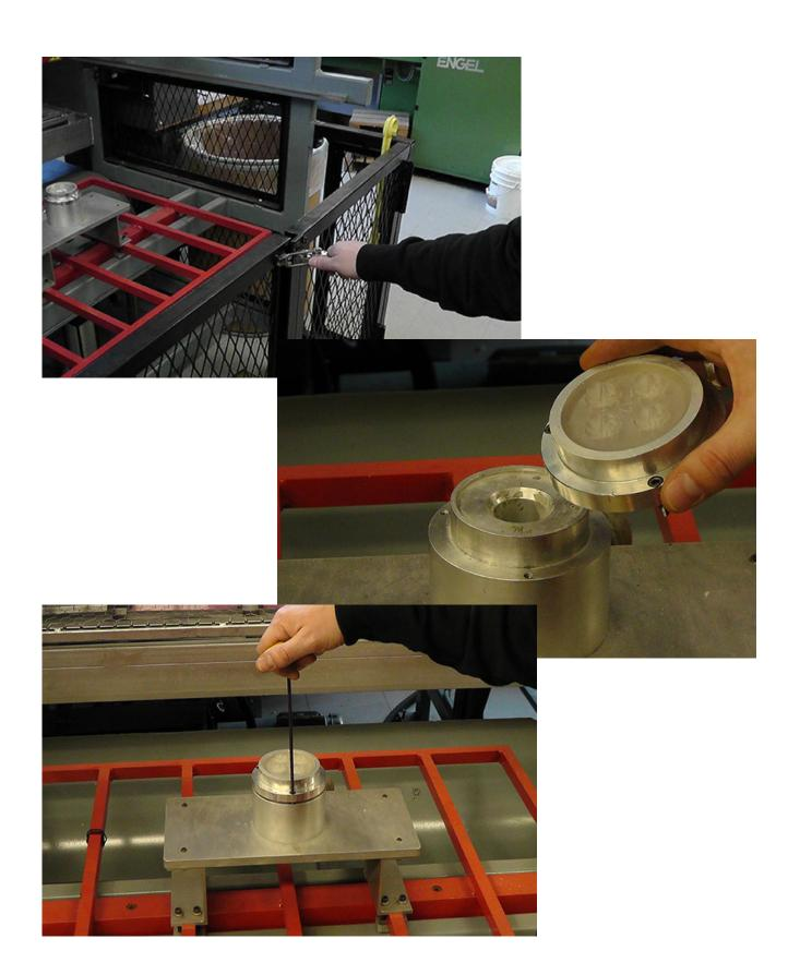
8. After die is secure, close the safety gate then press the INDEX MCF button to "off" and move the clamp system to its original position
