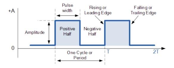
Leading/Trailing Edge Time: The leading (rising) edge time is defined as the time required for the pulse amplitude to rise from 10% threshold to 90% threshold; while the trailing (falling) edge time is defined as the time required for the pulse amplitude to fall from 90% threshold to 10% threshold as shown in the figure above.
