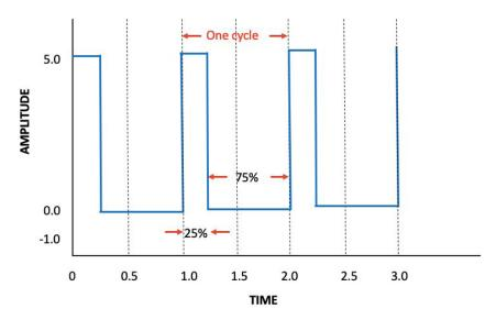
Symmetry: Symmetry is defined as the percentage that the rising period takes up in the whole period as shown in the figure below. This parameter is only available when ramp is selected.
