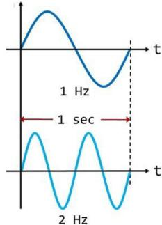
Period: This is the length of time in seconds that the waveform takes to repeat itself from start to finish. It is the reciprocal of frequency (T = 1/f)
