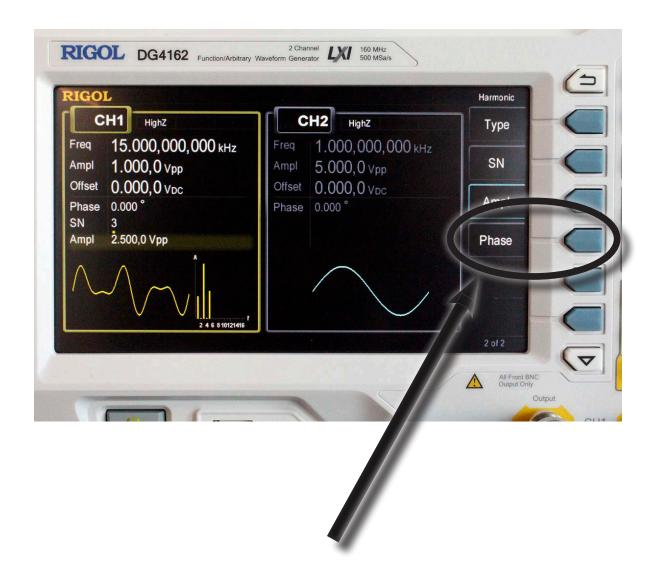
20. Use the numeric keypad to enter a value for the phase shift (i.e. 90°)
