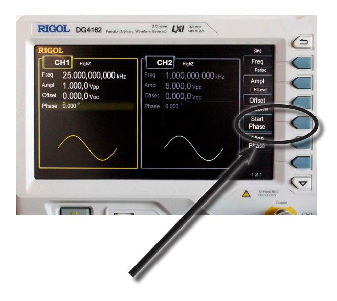
15. Use the numeric keypad to adjust the degrees of phase shift. (Use 0 if not needed).
