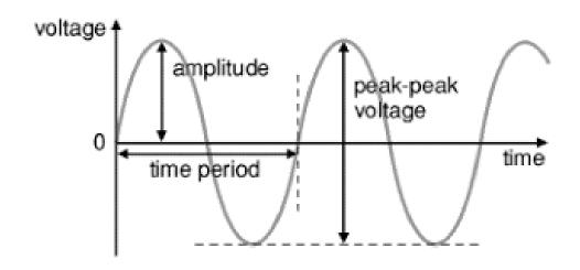
Amplitude: This is the magnitude or intensity of the signal waveform measured in volts or amps. This is often measured in peakto-peak voltage (Vpp), meaning, if the amplitude is 10Vpp, it has +5V and -5V.
