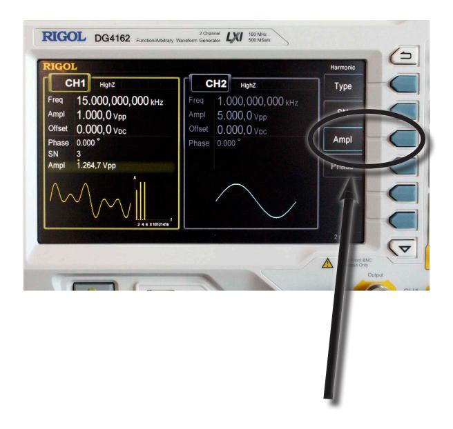
17. Use the numeric keypad to enter the amplitude value of the harmonic
