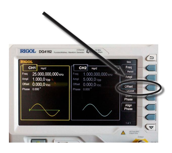
12. If a voltage offset is needed, use the numerical keypad to adjust the voltage offset. (Use 0 if no offset is needed)
