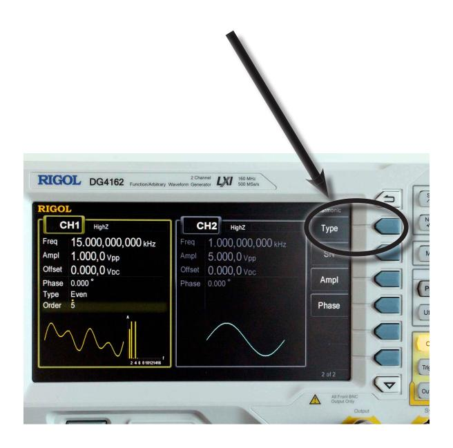
10. Press the appropriate softkey to set the harmonic type (i.e. Odd)
