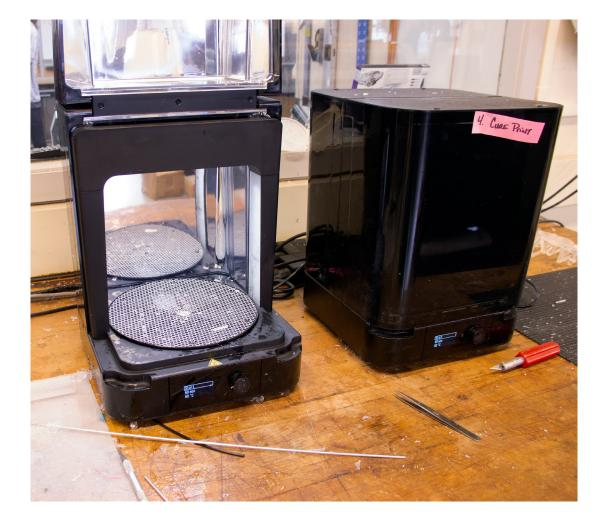
4. Close the door and use the selector dial to highlight START. Press the selector dial to begin curing
