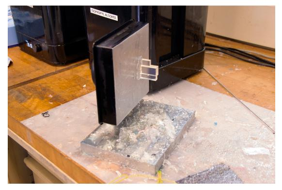
2. Remove the part from the build platform using the scrapper
