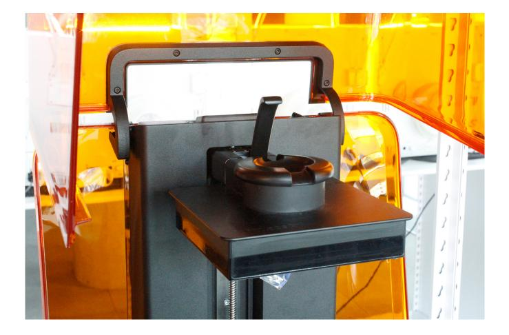
4. Pull the build platform directly towards you and immediately turn it over to prevent resin spills
