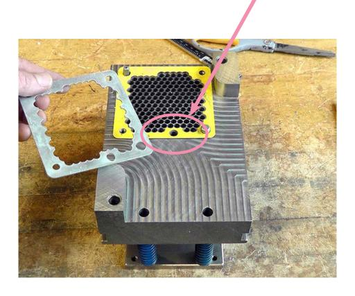
8. Install your core mold onto the MUD insert. Don't forget to snug your fasteners tightly!
