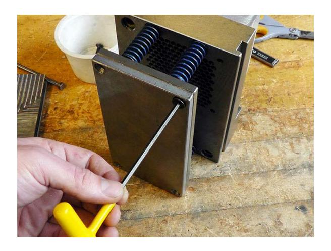
12. Prior to installing the MUD insert into the machine, lay it on the table to see how far the ejector pins might extend from the surface. You may need to re-measure your part and choose shorter ejector pins or increase the size of the shims
