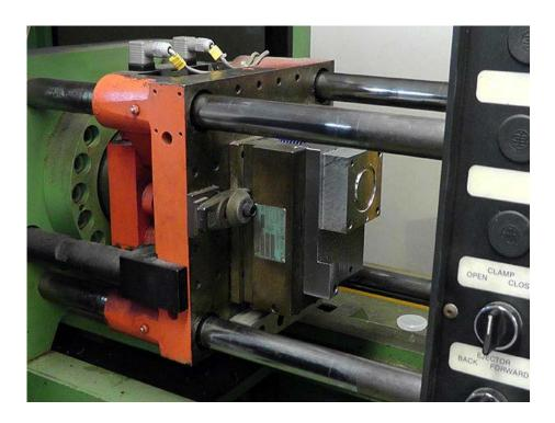
14. Don't forget to test your ejector pins on the machine! Look to make sure that all the pins extend and the sprue ejector pin has been installed and is extending also!!!
