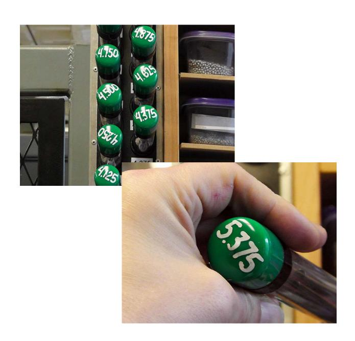
5. If the ejector pins are longer than (X + 3.892), use a shim or two!
