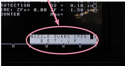
8. Press MOLD CLOSE Button on Controller Pendant. Again, make sure the screen says SETUP MODE!!! If it isnt in SETUP MODE, the mold will close very quickly and could crash.
