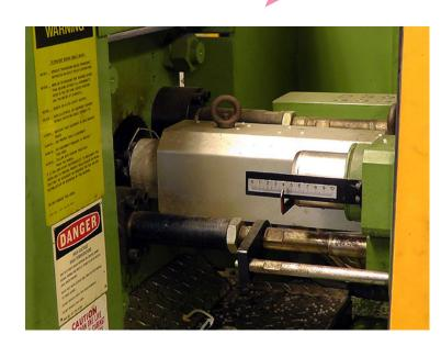
7. Retract the Nozzle and turn the INJECTION Switch to the INJECT position and extrude the Dyna-Purge from the nozzle
