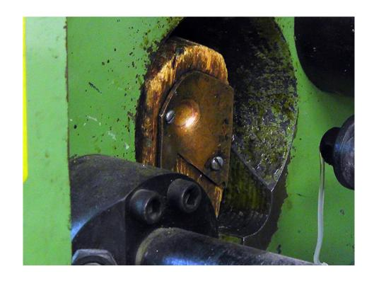
6. Turn the NOZZLE Switch to the FORWARD position until the Nozzle is pushing firmly against the wooden block and then turn the INJECTION Switch to the FEED position to fill the Nozzle with the Dyna-Purge
