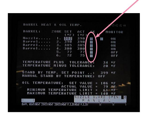
15. When the machine reaches operating temperature, retract the nozzle using the NOZZLE switch.
