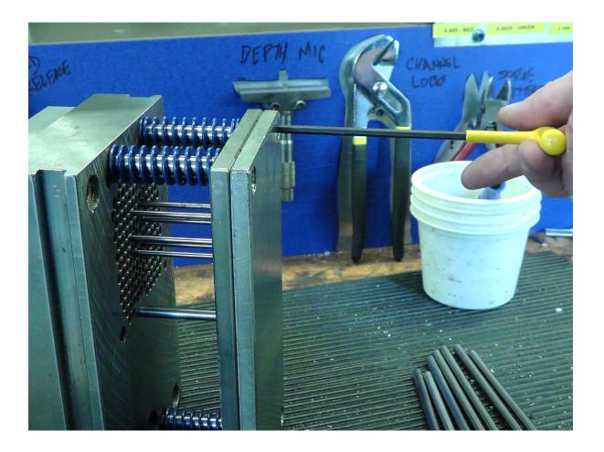
10. Install the large bolt onto the Core MUD insert
