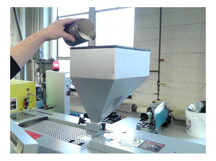
10. Extrude the clear resin until it no longer has any color by repeating step #7.
