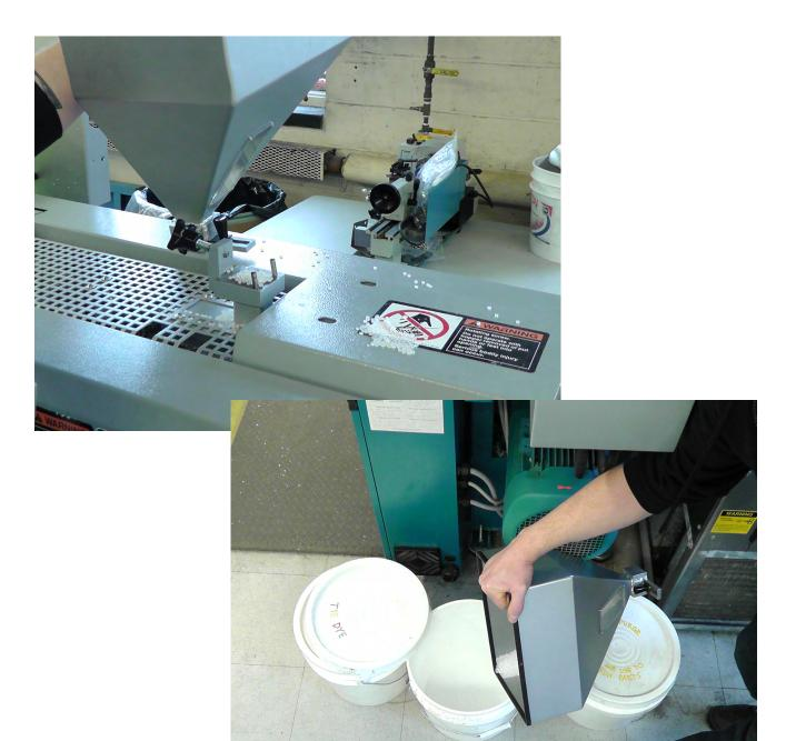
3. Replace the hopper (Remeber to tighten the bolt on the side!
