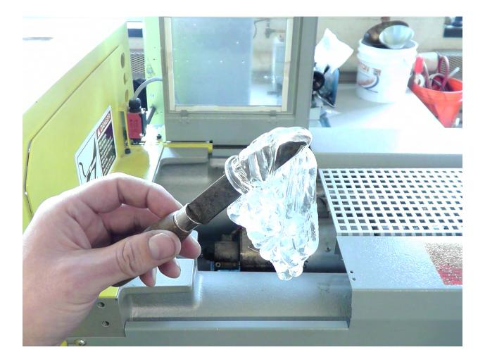
11. When the plastic is finally clear, go into the "Setup" mode by pressing and holding the (HAND) button for longer than 3 seconds (SEE STEP #12 IN MAIN GUIDE), then move PLASTICIZING UNIT back to operating position
