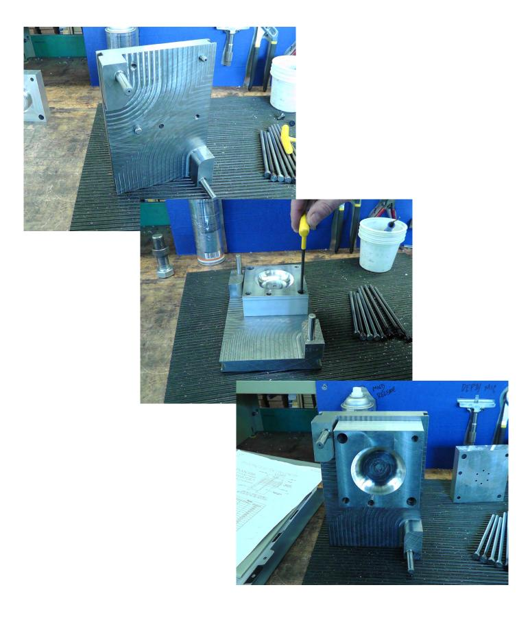
6. Install the Core mold on the MUD insert
